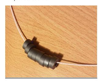
2. Make a 1<sup>st</sup> windings - 2 turns and put the coils like on the photo below:
