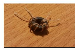
4. Remove the insulation with the wires; identify the ends of the wires and solder them to the main board.
