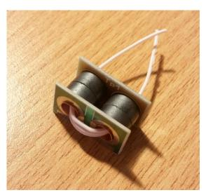
6. Put the soldered T2 to PCB and solder it at the 3 places.
