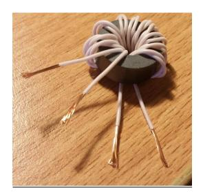
3. Using the tester - Identify the ends of the wires and merge the "Beginning of the wire 2 and the End of the wire 1"
