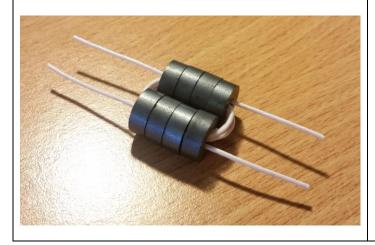
4. Put the transformer to PCB. Recommends add a hot glue for fixing the transformer on the board. Solder the ends of the windings according to the scheme
