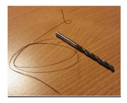
3. Put off the coil from the bit and make sure that is looks symmetrically and uniformly. Make the 2<sup>nd</sup> coil L2.
