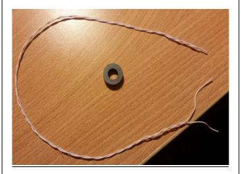
2. Make a winding - 10 turns by twisted wires. Remove the insulation.
