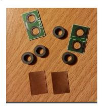
3. Merge two coils and put the cylinder's foil inside of the coils. The same procedure for the second 2 coils.
