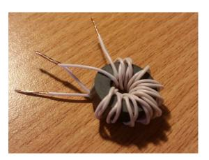
4. Put the coil to the main board. Solder the wires according to the scheme. Recommend to add a hot glue to fix the coil on the board.
