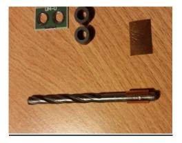
**4.** Construct the boards (see the picture below). The ends of the foil should be soldered to the PCB by the circle. (Coils are not soldered on the photo below!)
