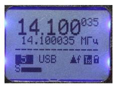
The synthesizer supports to display of two frequencies: Active frequency of VFO is displayed in large characters on the screen, the value of alternative frequency is indicated below, in smaller characters. Switching between frequencies by swap button SW4 "VFO A/B". In order to equalize the frequency of both values use the equal button SW8 "VFO A=B".
